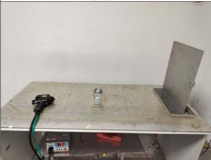
ESD Test Setup Photograph
