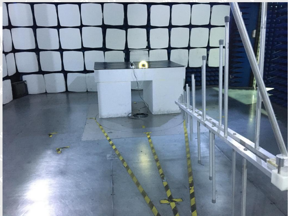
Radiation Emission Test View(30MHz to 1GHz)
