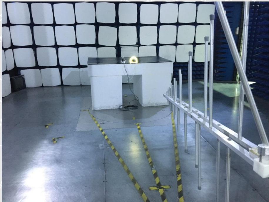
Radiation Emission Test View (30MHz~1000MHz)
