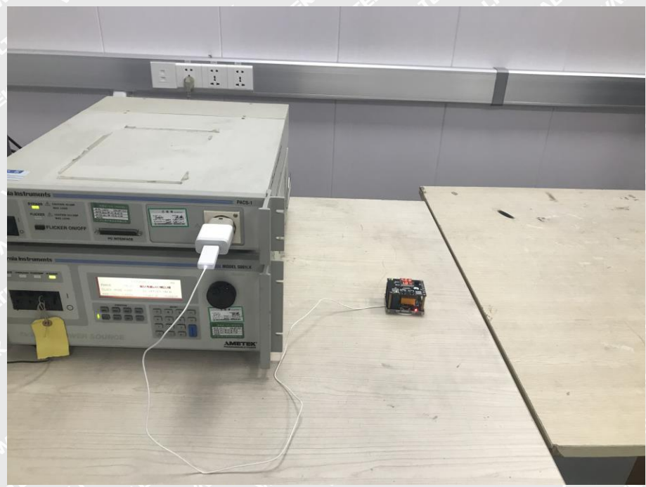
Harmonic/Flicker Test View
