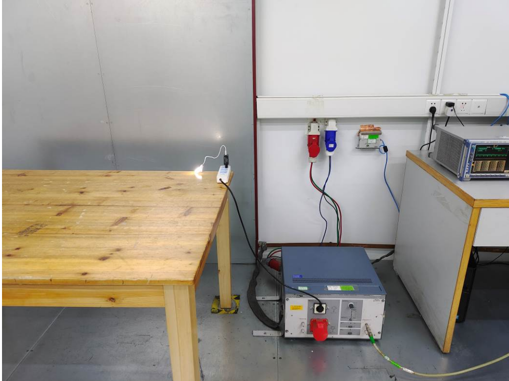
EN IEC 55015 RADIATED EMISSION TEST SETUP
