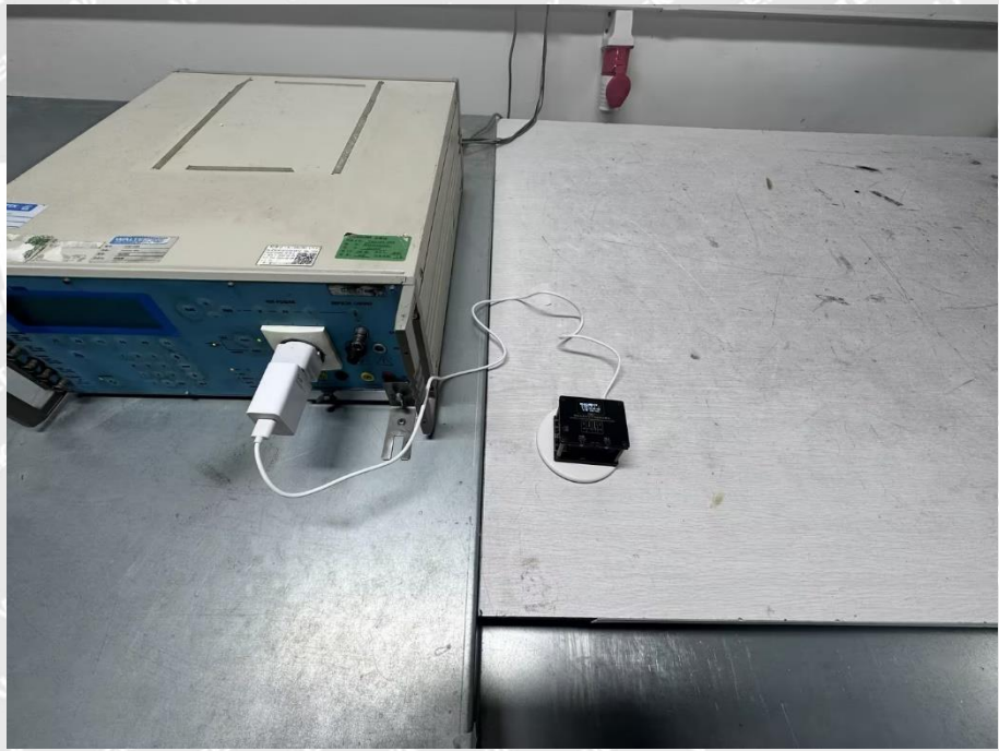
EFT/ Surges/ Dips and Interruptions Test View
