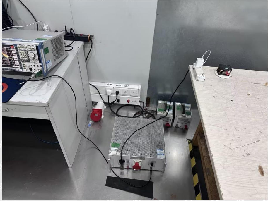
Conducted Emission Test Setup
