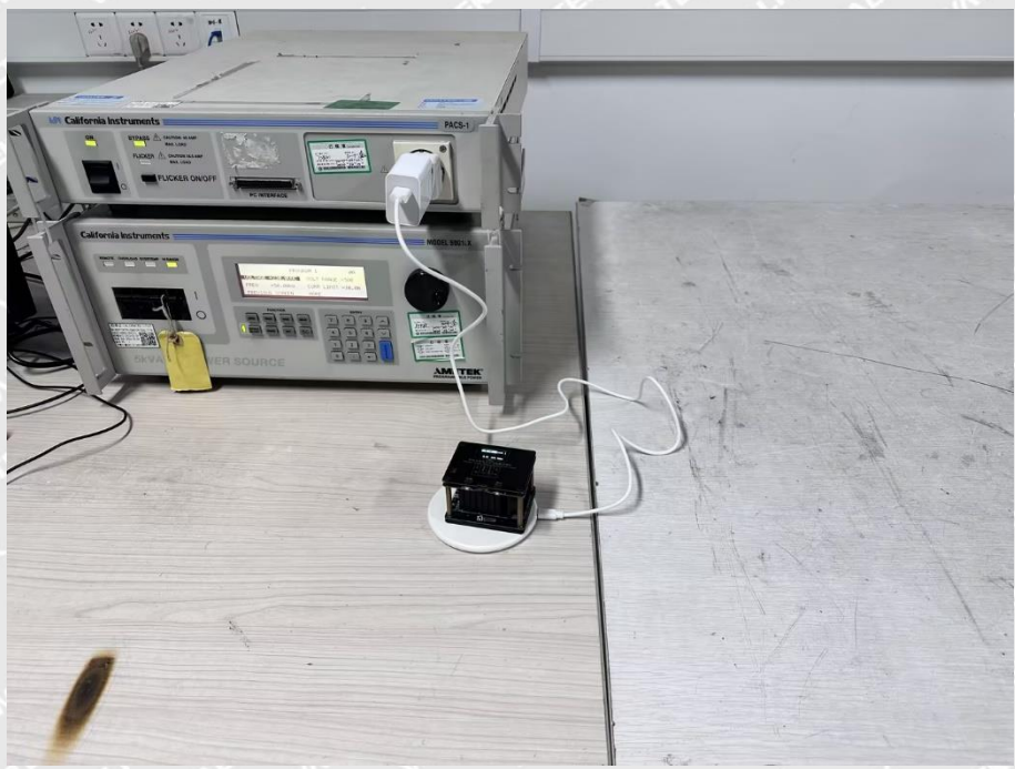
Harmonic/Flicker Test View
