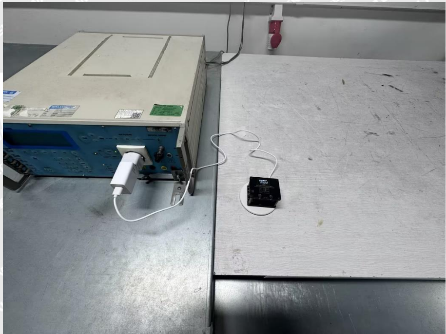
EFT/ Surges/ Dips and Interruptions Test View
