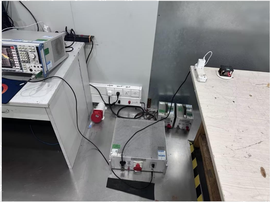
Conducted Emission Test Setup
